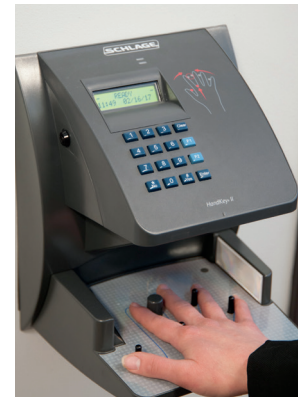
Safe deposit hand scanner
